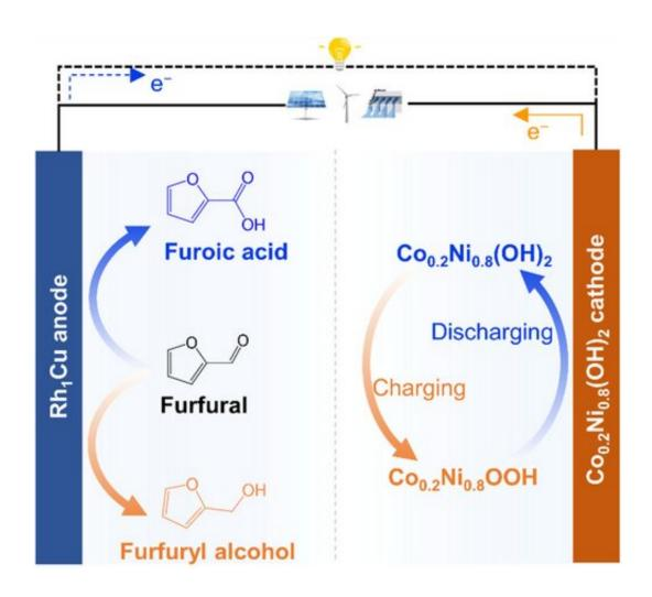
A rechargeable biomass battery was designed to integrate electricity storage/generation and electrosynthesis of useful chemicals from furfural in one system. By electrocatalyst (Rh1Cu single-atom alloy) and cathode redox pair (Co<sub>0.2</sub>Ni<sub>0.8</sub>(OH)<sub>2</sub>) design, the battery produces furfuryl alcohol in charging process and produces furoic acid in discharging process, reaching a high open circuit voltage of 1.29 V and power density of 107 mW cm<sup>-2</sup>. Credit:
