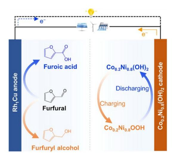
A rechargeable biomass battery was designed to integrate electricity storage/generation and electrosynthesis of useful chemicals from furfural in one system. By electrocatalyst (Rh1Cu single-atom alloy) and cathode redox pair  $(Co_{0.2}Ni_{0.8}(OH)_2)$  design, the battery produces furfuryl alcohol in charging process and produces furoic acid in discharging process, reaching a high open circuit voltage of 1.29 V and power density of 107 mW cm<sup>-2</sup>. Credit:
