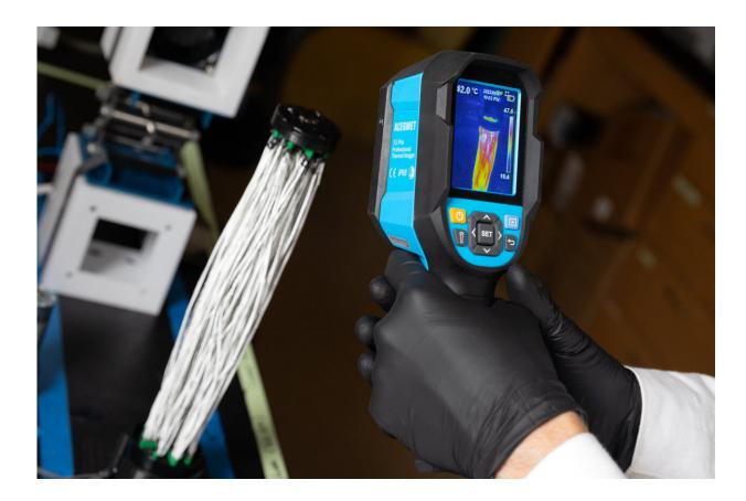
A thermal imaging device shows heat distribution in sorbent-coated carbon fibers that are the key component of a cheaper-to-build, more efficient direct air capture system proposed by Georgia Institute of Technology researchers. Credit: Candler Hobbs, Georgia Institute of Technology
