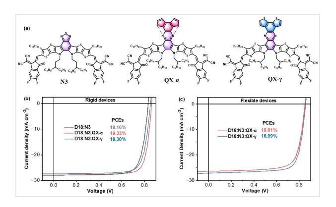
The molecular structures of N3, QX- $\alpha$ , and QX- $\gamma$  (a); J-V curves of the rigid (b) and flexible (c) organic solar cells. Credit: NIMTE
