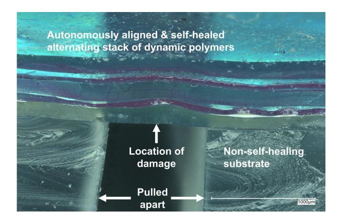
A depth-profiled digital microscope photograph of a 5-layer alternating laminate film of immiscible dynamic polymer films which have been damaged, autonomously aligned, self-healed and then pulled apart on a non-self-healing subject (to show the location of the damage). Credit: Bao Group, Stanford U.
