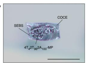
Fibers with different cross-sectional areas filled with a magnetic elastomer composite. Fibers with cross-sectional areas of (a)  $1000 \times 500 \ \mu m^2$  and (b)  $500 \times 200 \ \mu m^2$ . Scale bar =  $500 \ \mu m$ . Credit: *Advanced Materials* (2023). DOI: 10.1002/adma.202301916
