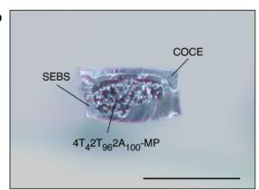
Fibers with different cross-sectional areas filled with a magnetic elastomer composite. Fibers with cross-sectional areas of (a)  $1000 \times 500 \,\mu\text{m}^2$  and (b)  $500 \times 200 \,\mu\text{m}^2$ . Scale bar =  $500 \,\mu\text{m}$ . Credit: *Advanced Materials* (2023). DOI: 10.1002/adma.202301916
