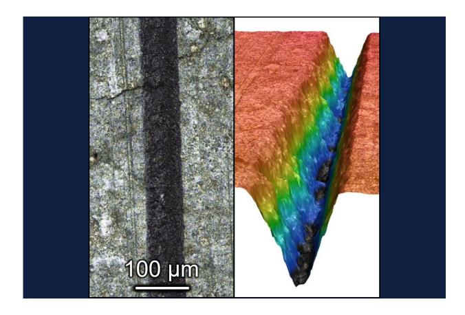
The team used laser-engraved microchannels to improve flow within their new electrodes. Pictured are views of a single microchannel from above, left, and the side, right. Credit: Smith research group, University of Illinois Urbana-Champaign
