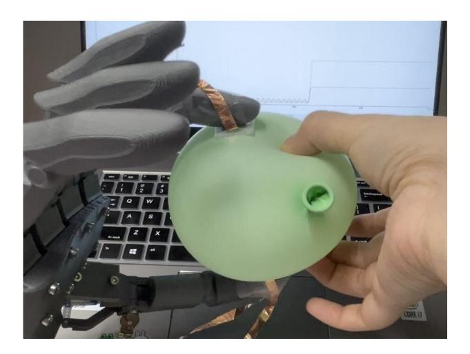
Testing the iontronic sensor's ability of tactile sensing via a robotic hand and a balloon. Credit: Cheng Group
