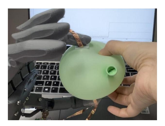
Testing the iontronic sensor's ability of tactile sensing via a robotic hand and a balloon. Credit: Cheng Group
