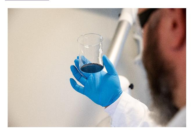
The batteries are recycled to produce a powder, or "black mass", made up of nickel, manganese, cobalt, lithium and graphite.
