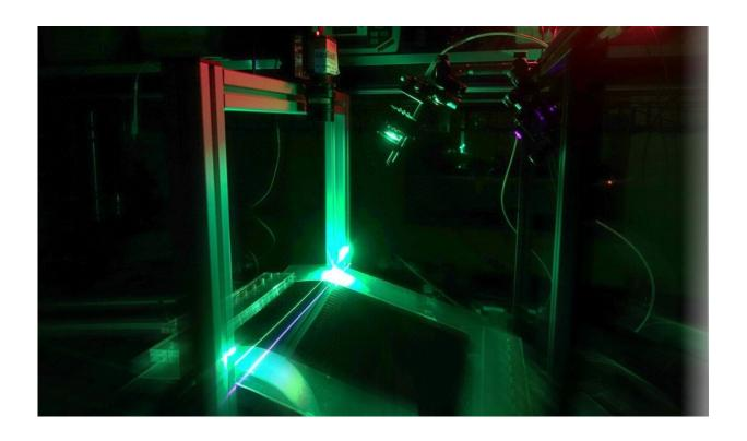
Using artificial intelligence and optical measurement technology, SURFinpro detects, classifies and visualizes defects in real time as the process is ongoing. Credit: Fraunhofer-Gesellschaft
