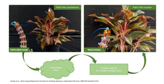
The robot explores the workspace through plant-like oscillations to gather information from the environment and build a knowledge base. By mean of a greedy search approach, the robot can identify the point of interest and implements reaching through plant-like tropism. Credit: Donato et al
