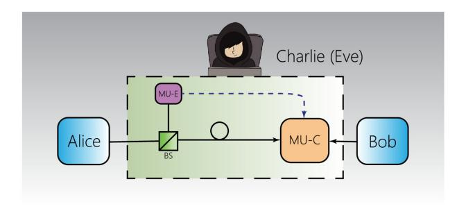
Schematic diagram of our tagged method. MU-E, the measurement unit for projecting Alice's states on the Z basis; MU-C, the measurement unit for BSM; BS, beam splitter. Credit: *Optica* (2023). DOI: 10.1364/OPTICA.485389
