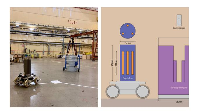
The neutron-detecting robot maneuvering through a large space, left, with a schematic of the robot and its target, right. Credit: Eric Lepowsky
