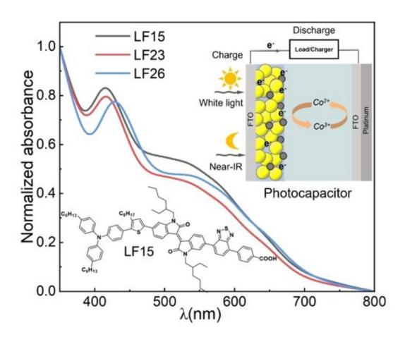
The simple single-component photocapacitor can be charged by both day-orroom light and near-IR radiation. Among isoindigo dyes, LF15 with rigid benzoic acid as the anchor group exhibits superior photoelectric performance compared to Z-cyanoacetic acid-anchored LF23 and LF26. Credit: *Chemistry – An Asian Journal* (2023). DOI: 10.1002/asia.202300188
