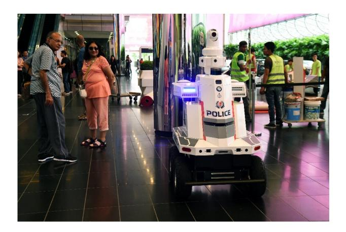
The robots are equipped with cameras, sensors, speakers, a display panel, blinkers and a siren.
