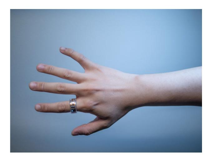
The OmniRing doesn't have a display and so can support a longer battery life. This makes it possible to wear the ring all the time, including while sleeping and swimming, enabling the ring to capture deeper and more intimate levels of sensing information. Credit: Taiting Lu
