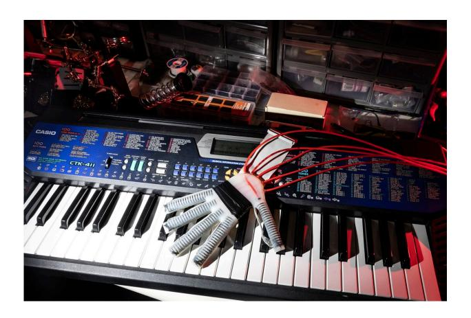
The soft robotic glove integrates five actuators into a single wearable device that conforms to the user's hand. Credit: Alex Dolce, Florida Atlantic University
