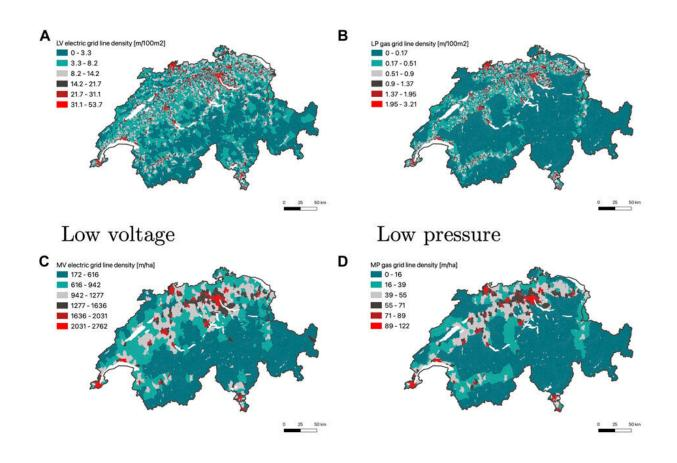
Map of Switzerland with the grid line density estimation using the equidistant method (Eqs 2, 4). (A,C,E) show the electric grid polygons. (B,D,F) display the equivalent pressure gas grid Voronoi polygons, within a range of 5 km around the EHP and HP gas grid lines. Credit: *Frontiers in Energy Research* (2023). DOI: 10.3389/fenrg.2023.1164813
