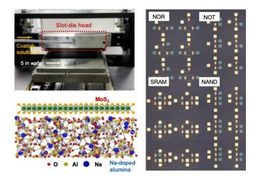
Photograph of the slot-die machine to coat dielectric and semiconducting layers over 5-inch wafer. Schematic illustration of a semiconducting MoS<sub>2</sub> layer and a Na-doped alumina layer as a dielectric. Various logic gates demonstrated including NOR, NOT, SRAM, and NAND. Credit: Kwon et al
