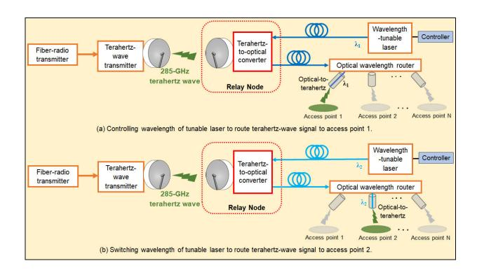
Concept of transparent relay and switching of terahertz-wave signals using direct terahertz-optical conversion and optical wavelength control. Credit: National Institute of Information and Communications Technology (NICT), Sumitomo Osaka Cement Co., Ltd., Nagoya Institute of Technology, and Waseda University
