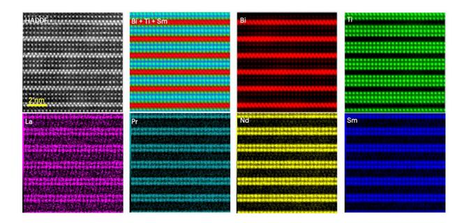
Atomically resolved elemental mappings for the film of x = 1.5, including HAADF images along [11<sup>-0</sup>] zone axes, superimposing Bi + Ti + Sm mapping and individual distribution of Bi, Ti, La, Pr, Nd and Sm elements. Credit: Yang et al
