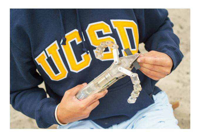
The robot is equipped with flipper-like appendages which allow it to swim under sand. The two black fins on its nose ensure that it remains submerged under the sand. Credit: David Baillot/University of California San Diego
