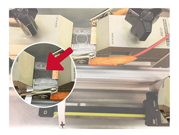
UH researchers stretching, testing and monitoring the stretchable fabric-based lithium-ion battery's performance. The gray striated section is the battery prototype. Credit: University of Houston
