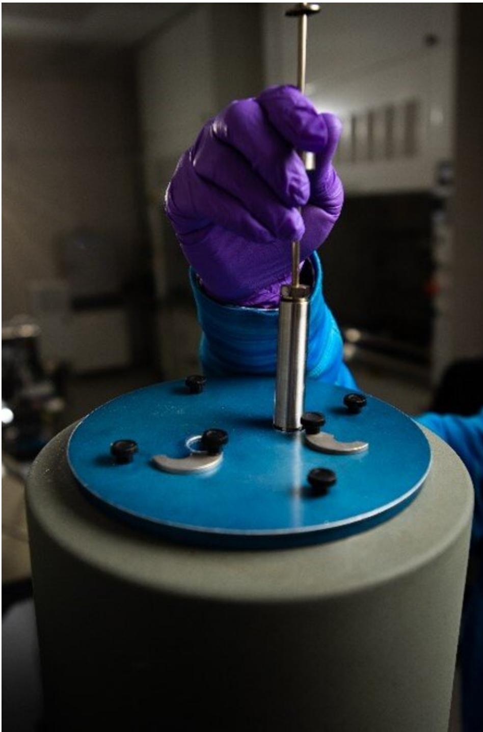
The Flipper mixes chemicals by rotating upside down with samples secured. Credit: Andrea Starr | Pacific Northwest National Laboratory
