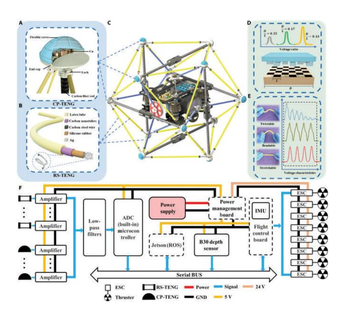
Construction diagram and applications of TENG based tensegrity . (A and B) Basic structures of the CP-TENG sensor (A) and RS-TENG sensor (B). (C)
