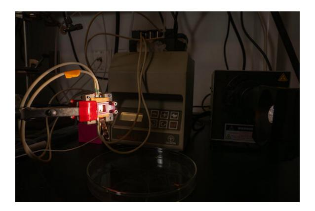
A photoreactor developed by Rice University's Mohite research group and collaborators achieved a 20.8% solar-to-hydrogen conversion efficiency. Credit: Gustavo Raskoksy/Rice University
