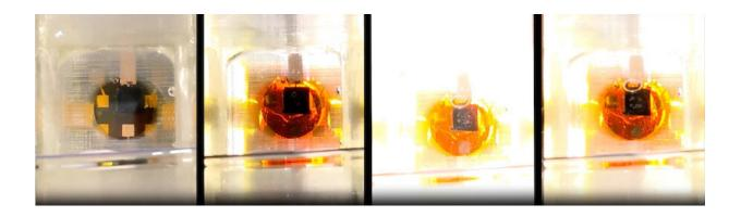
Series of four still images from a sample video showing how a photoreactor from Rice University splits water molecules and generates hydrogen when stimulated by simulated sunlight. Credit: Mohite lab/Rice University
