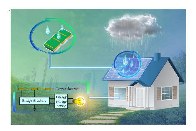
This diagram shows what these D-TENG panels might look like. It also illustrates how the bridge structure, when combined with the lower electrodes, can lead to improved energy storage. Credit: iEnergy, Tsinghua University Press
