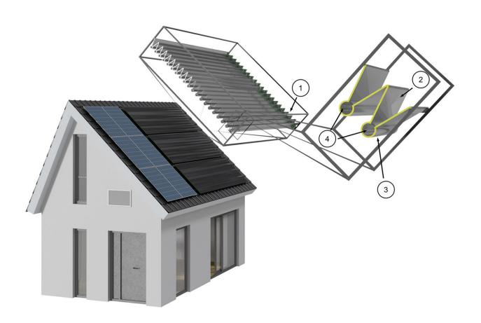
Potential application of the proposed low-cost, high-efficiency photoreactors on the roof top of a low-energy house. Credit: *Joule* (2023). DOI: 10.1016/j.joule.2023.05.006
