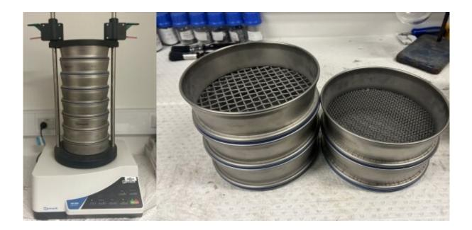
The new patented PV recycling process developed at UNSW involves crushing and sieving material inside a vibrating container for around 5–15 minutes. Credit: Professor Yansong Shen
