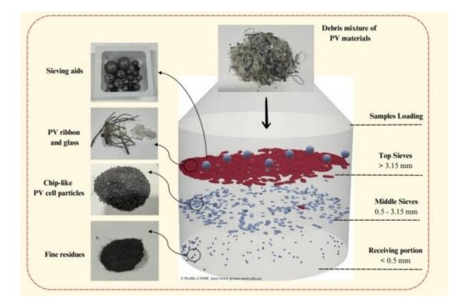
The new patented recyling process from researchers at UNSW uses sieving aids to more effectively separate the material that makes up a solar panel, allowing valuable elements such as silver to be recovered and reused. Credit: Professor Yansong Shen
