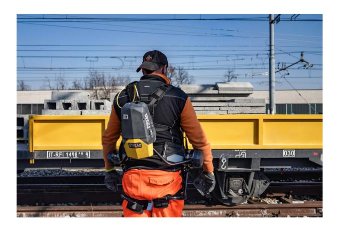
The STREAM exoskeleton (StreamEXO) generates forces which are distributed to the shoulders and legs to support the worker's back during handling activities, such as lifting and carrying heavy loads. The device's ergonomics have been studied to enhance comfort and provide totally free movements, ensuring a perfect fit on the worker's body while carrying out dynamic activities. Credit: IIT-Istituto Italiano di Tecnologia
