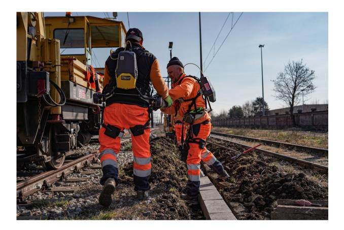
The StreamEXO prototype was validated in approximately 100 hours of use by 15 people during a 6-month test campaign hosted in Italy highlighting a 50% reduction in the ergonomic risk of physical overload and a 30% of muscle fatigue. The design of the StreamEXO created by IIT was intended to be a comfortable solution to be used during work shifts for workers employed in the
