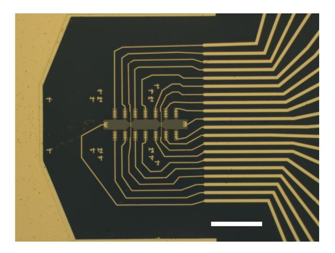
Quantum point contact device in Strontium Titanate. Scale bar length is 100 microns. Credit: Evgeny Mikheev et al
