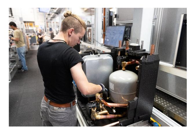
At the Bosch Home Comfort Group plant, heat pump interior units are carefully put together.
