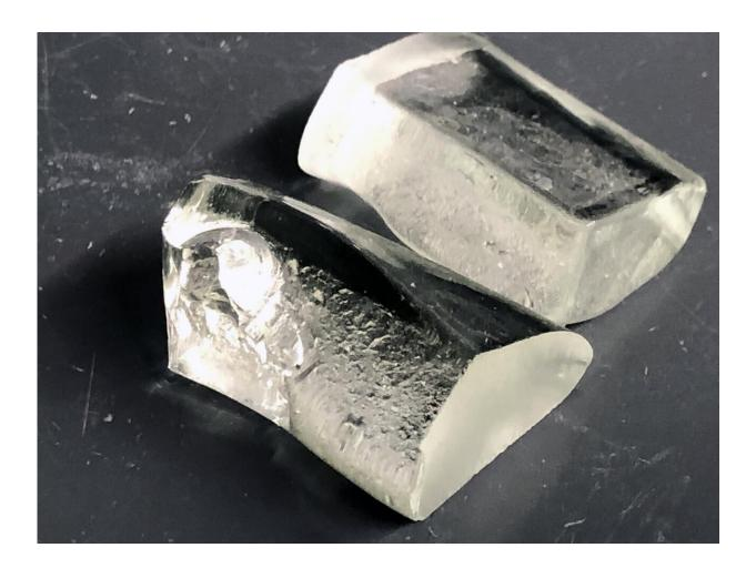
A sample of LionGlass, a new type of glass engineered by researchers at Penn State that requires significantly less energy to produce and is much more damage resistant than standard soda lime silicate glass. Credit: Adrienne Berard / Penn State. <u>Creative Commons</u>
