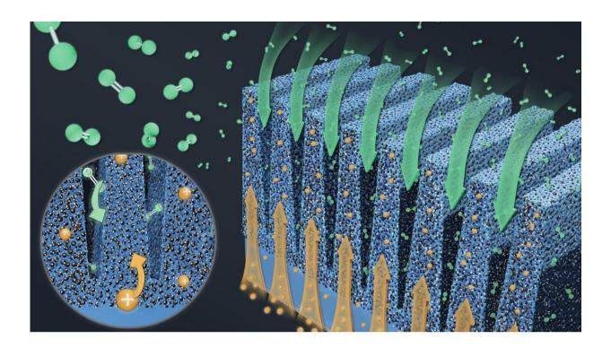
The grooved electrode design enables the transport of oxygen and protons to be partitioned into separate grooves and ridges, respectively, enabling faster movement of both species, and hence higher fuel cell performance. Credit: *Nature Energy* (2023). DOI: 10.1038/s41560-023-01263-2
