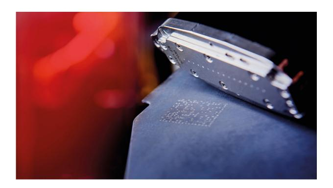
Data matrix code on hot-formed sheet metal, printed using industrial printer Credit: © Senodis Technologies GmbH
