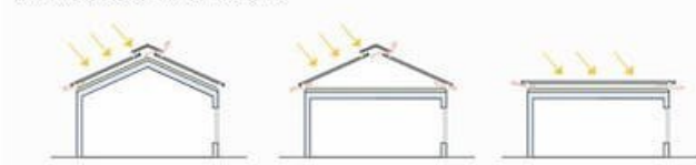
Ventilated and reflective roofs
