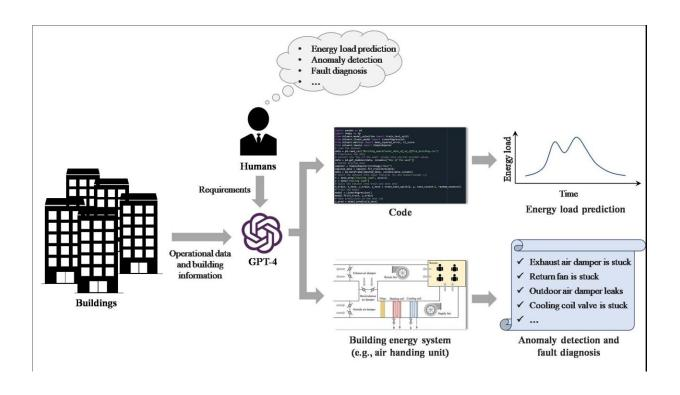
How the GPT-4 works on automated data mining for building energy management. Credit: Chaobo Zhang, Jie Lu, Yang Zhao
