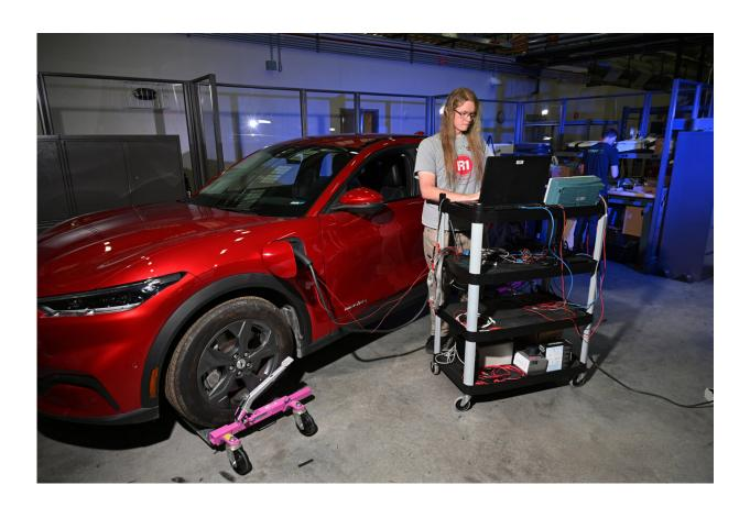
INL intern, Jake Guidry, is using the AcCCS system to interface with an electric vehicle through the CCS charge port to evaluate the cybersecurity posture of the charging communication protocols. Credit: Idaho National Laboratory
