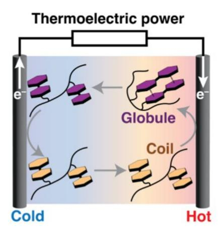
Diagram of phase transitions in the thermocell: This diagram illustrates the polymer phase transitions of the modified PNIPAM hydrogel, showing how the polymer elongates into a coil and dissolves at low temperatures, and curls up into a globule and becomes solid at high temperatures. When used as a thermocell battery, temperatures above 25 degrees Celsius generated a voltage. Credit: 2023 Zhou et al. CC-BY
