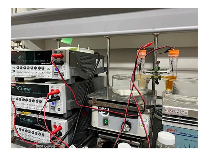
Experimental thermocell setup: Electrochemical refrigeration is currently not generally used or commercialized due to its low performance compared with other options, such as electrical refrigeration. However, this research may change that. Credit: 2023 Yamada CC-BY
