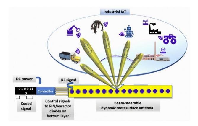
A conceptual depiction of the application of a beam-steerable DMA for Industrial IoT applications. Credit: *Research*
