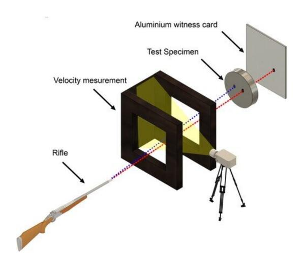
The attack and rear faces of the perforated plates were photographed. Pass and fail shots were selected from each plate and sectioned parallel and across the penetration direction for further examination. Credit: *Materials Science and Technology* (2023). DOI: 10.1080/02670836.2023.2229175
