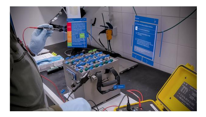
Carrying out a battery test with guided resistance measurement in the workshop. Credit: © Fraunhofer FKIE
