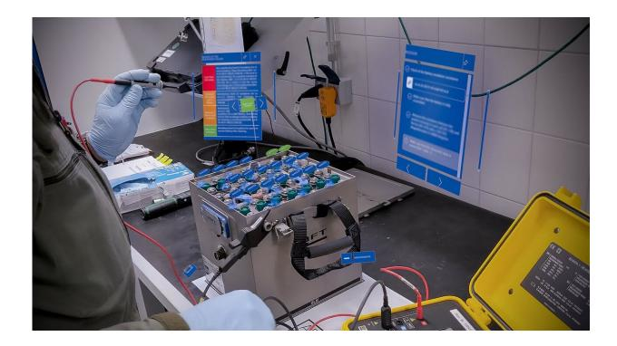
Carrying out a battery test with guided resistance measurement in the workshop. Credit: © Fraunhofer FKIE
