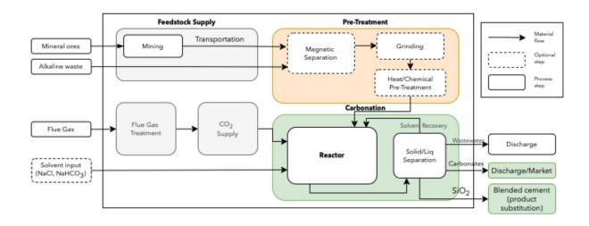
Direct carbonation system boundaries. Mineral ores refer to naturally-occurring and exploitable magnesium and calcium sources (serpentine, wollastonite and olivine). Alkali waste treatment depends on the feedstock source with magnetic separation and heat pre-treatment being optional. Credit: *Energy & Environmental Science* (2023). DOI: 10.1039/D3EE01803B
