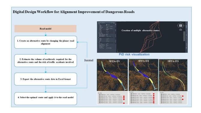
from the creation of BIM models for roads to the generation of optimal alternatives to minimize the risk of traffic accidents. Credit: Korea Institute of Civil Engineering and Building Technology
