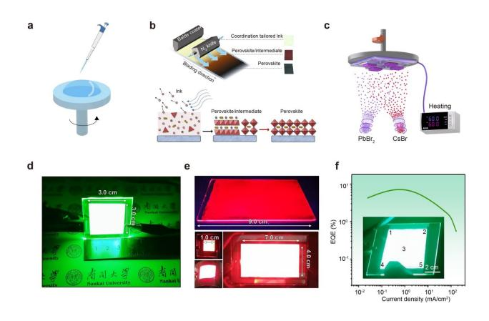
(a), blade-coating (b), and vapor deposition (c); Large-area PeLED devices based on spin-coating (d), blade-coating (e), and vapor deposition (f). Credit: Changjiu Sun, Yuanzhi Jiang, Keyu Wei, Mingjian Yuan
