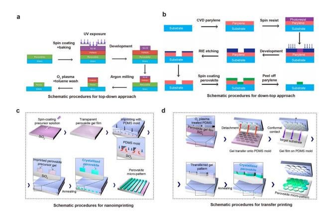
Top-down (a) and down-top (b) lithography steps for patterned perovskite arrays; nanoimprinting (c) and imprinting-transfer printing (d) steps for patterned perovskite arrays. Credit: Changjiu Sun, Yuanzhi Jiang, Keyu Wei, Mingjian Yuan
