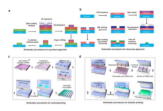
Top-down (a) and down-top (b) lithography steps for patterned perovskite arrays; nanoimprinting (c) and imprinting-transfer printing (d) steps for patterned perovskite arrays. Credit: Changjiu Sun, Yuanzhi Jiang, Keyu Wei, Mingjian Yuan
