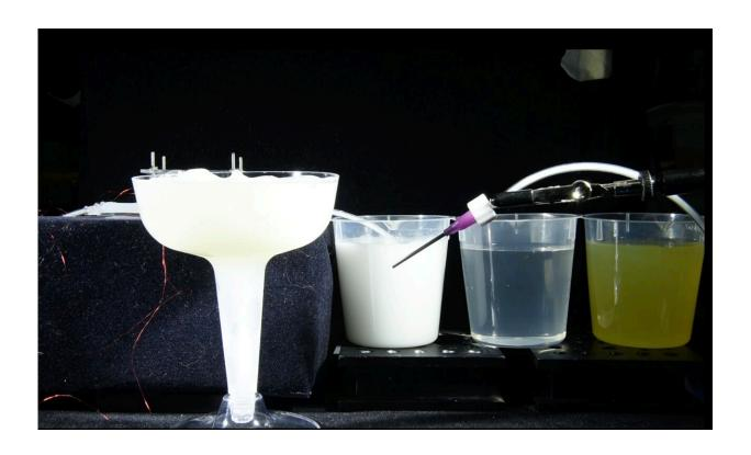
A compact, soft pump with adjustable pressure flow is versatile enough to pump a variety of fluids with varying viscosity, including gin, juice, and coconut milk. Credit: Harvard Microrobotics Lab/Harvard SEAS
