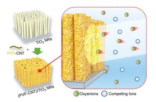
Schematic diagram of (left) the formation of  $(PVF-CNT)/TiO_2$  NR electrodes. PVF-functionalized CNT was deposited on the NR arrays by electrodeposition. (Right) The proposed solar-driven PEC separation of heavy metal oxyanions is displayed. Credit: *Small* (2023). DOI: 10.1002/smll.202305275
