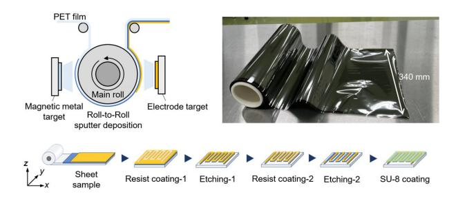
Making films: The roll-to-roll sputter deposition manufacturing technique is well established and can create etchable films in large quantities for use in commercial settings. Credit: Tanaka et al CC-BY-ND
