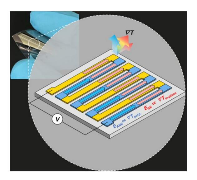
Making tracks: By etching the circuits in a special alternating pattern, undesirable effects are reduced that would otherwise impede the circuits' ability to produce usable data. Credit: Tanaka et al CC-BY-ND
