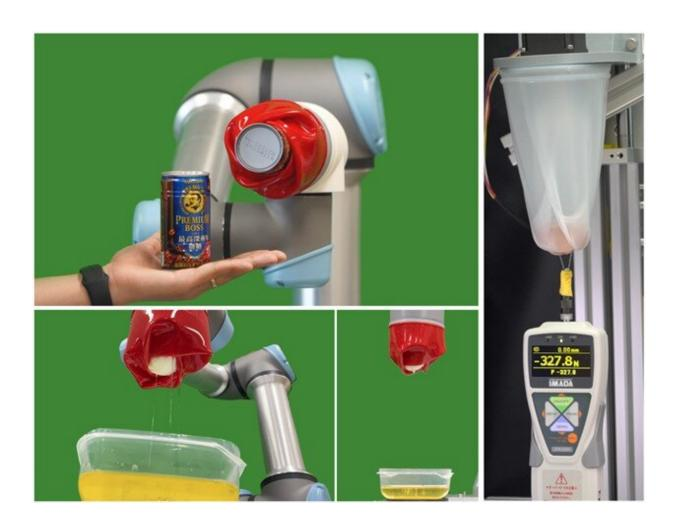
ROSE can pick up a wide variety of objects with ease. The top-left image shows it grasping a coffee can, whereas the bottom images show it successfully picking up a peeled chicken egg submerged in olive oil. The image on the right shows the maximum lifting force that ROSE can withstand. Credit: Van Anh Ho from JAIST.
