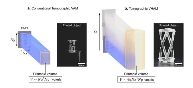
Increasing the number of printed voxel generated from the same DMD. a Conventional tomographic volumetric additive manufacturing. b Tomographic volumetric helical additive manufacturing. Scale bars: 10 mm. Credit: *Light: Advanced Manufacturing* (2023). DOI: 10.37188/lam.2023.012
