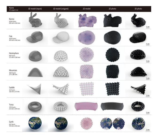
The software the team created is based on an important algorithm in the field of origami. It can decompose a 3D input object and output a 2D pattern. This process would take a human artist time, patience and a lot of trial and error. This algorithm is what first inspired the team to explore the idea of rapid 4D fabrication and is fundamental to the process. Credit: ©2023 Narumi et al. CC-BY-ND
