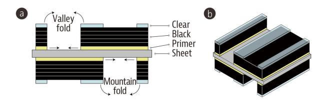
In origami, there are two main types of creases used: valley folds and mountain folds. In each case, the paper is folded either inwards or outwards. To make these folds, gaps are left on one side of the heat-shrink sheet to allow for that part of the sheet to fold inwards, like a valley, or outwards, like a mountain, when heat is applied. Credit: ©2023 Narumi et al. CC-BY-ND
